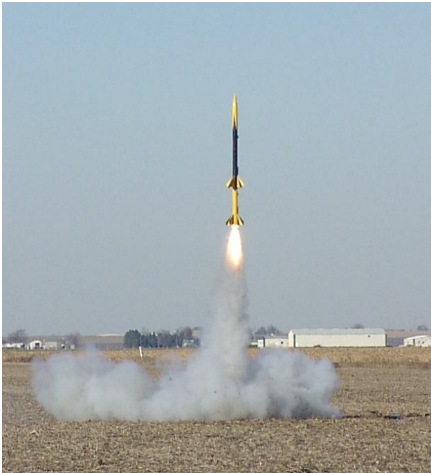
Greg Smith's Quantum Leap boosts on an H242 at Flatville on November 13, 2004. The upper stage had a G80. Unfortunately the payload section separated at staging and the rocket did loop-the-loops. The booster stage then landed on some power lines. It sure looked good taking off though. Photo by Greg Smith.
