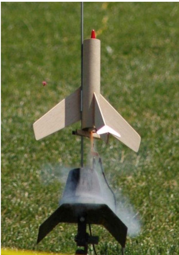
Jonathan Sivier's Centuri Mach 10 ignites at GARLO 2005. You can see the igniter plug flying away to the right of the rocket after bouncing off the blast deflector. Photo by Corwin Carroll.
